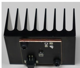
Picture 4. Fins facing vertical (Nichia uses this orientation)
